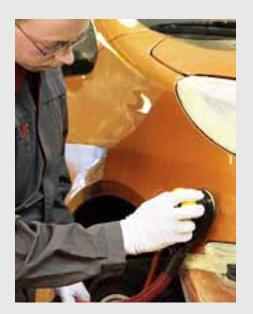
**FAST AND EFFECTIVE.** With Abranet dust-free effective sanding can be carried out during the entire process, from filler sanding to final polishing. This saves time and guarantees better quality.
