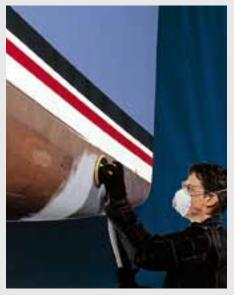
**LUNG PROTECTION.** Thanks to Abranet, a worker's lungs are now only exposed to a much smaller amount of dust. With a good dust extraction unit, special metals like zinc and aluminium or composites like carbon fibre and fibre glass can also be sanded.
