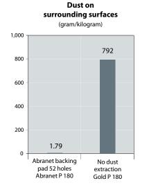
**TEST WINNER.** Laboratory tests show that Abranet has solved the dust problem. The amount of dust in the air when machine sanding with Abranet is 6,900 times less than when sanding using traditional abrasives without dust extraction.
