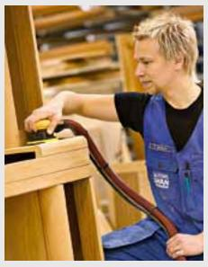
**BETTER CONTROL.** Dust-free sanding enables better control over sanding work. Many different tasks can be made simultaneously in the same room. And there will be less tidying up afterwards.
